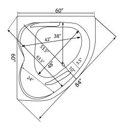
**NOTE:** Graphics may not be to scale. Specifications and features are subject to change without notice and are ± .25". All final measurements should be taken from **tub on site.** Access 18"x 18" or larger is required for each pump. Some pump locations and plumbing may extend beyond the perimeter of the bath.
