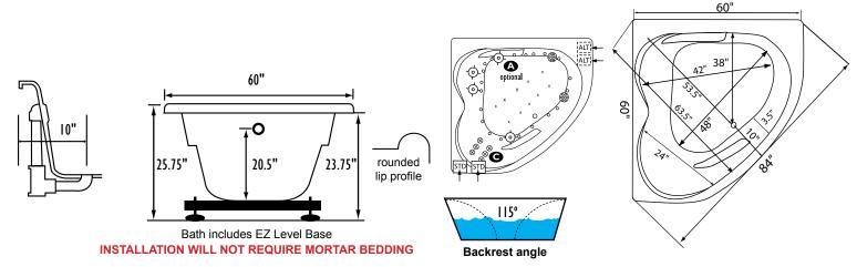
NOTE: Graphics may not be to scale. Specifications and features are subject to change without notice and are ± .25". All final measurements should be taken from tub on site. Access 18"x 18" or larger is required for each pump. Some pump locations and plumbing may extend beyond the perimeter of the bath.
