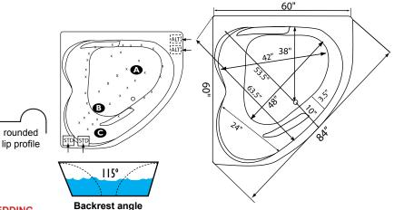
NOTE: Graphics may not be to scale. Specifications and features are subject to change without notice and are ± .25". All final measurements should be taken from tub on site. Access 18"x 18" or larger is required for each pump. Some pump locations and plumbing may extend beyond the perimeter of the bath.
