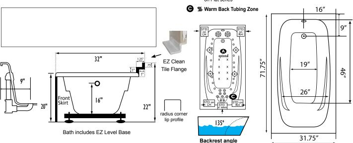
**NOTE:** Graphics may not be to scale. Specifications and features are subject to change without notice and are ± .25". All final measurements should be taken from **tub on site.** Access 18"x 18" or larger is required for each pump. Some pump locations and plumbing may extend beyond the perimeter of the bath.
