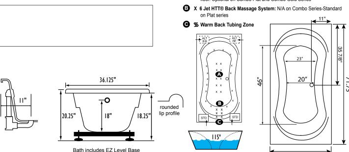
NOTE: Graphics may not be to scale. Specifications and features are subject to change without notice and are ± .25". All final measurements should be taken from tub on site. Access 18"x 18" or larger is required for each pump. Some pump locations and plumbing may extend beyond the perimeter of the bath.
