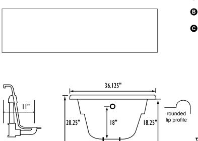
Bath includes EZ Level Legs **INSTALLATION WILL NOT REQUIRE MORTAR BEDDING**
