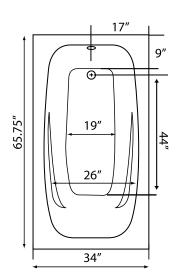
NOTE: Graphics may not be to scale. Specifications and features are subject to change without notice and are ± .25". All final measurements should be taken from tub on site. Access 18"x 18" or larger is required for each pump. Some pump locations and plumbing may extend beyond the perimeter of the bath.
