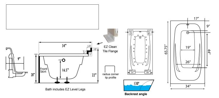
**NOTE:** Graphics may not be to scale. Specifications and features are subject to change without notice and are ± .25". All final measurements should be taken from **tub on site.** Access 18"x 18" or larger is required for each pump. Some pump locations and plumbing may extend beyond the perimeter of the bath.
