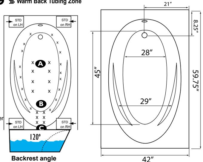
**NOTE:** Graphics may not be to scale. Specifications and features are subject to change without notice and are ± .25". All final measurements should be taken from **tub on site**. Access 18"x 18" or larger is required for each pump. Some pump locations and plumbing may extend beyond the perimeter of the bath.
