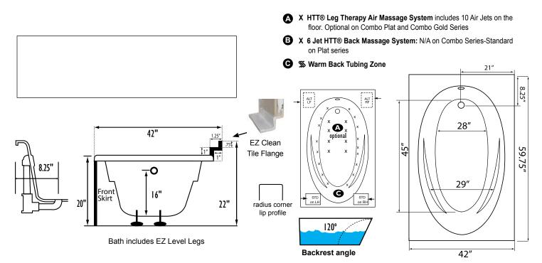
**NOTE:** Graphics may not be to scale. Specifications and features are subject to change without notice and are ± .25". All final measurements should be taken from **tub on site.** Access 18"x 18" or larger is required for each pump. Some pump locations and plumbing may extend beyond the perimeter of the bath.
