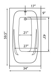
NOTE: Graphics may not be to scale. Specifications and features are subject to change without notice and are ± .25". All final measurements should be taken from tub on site. Access 18"x 18" or larger is required for each pump. Some pump locations and plumbing may extend beyond the perimeter of the bath.
