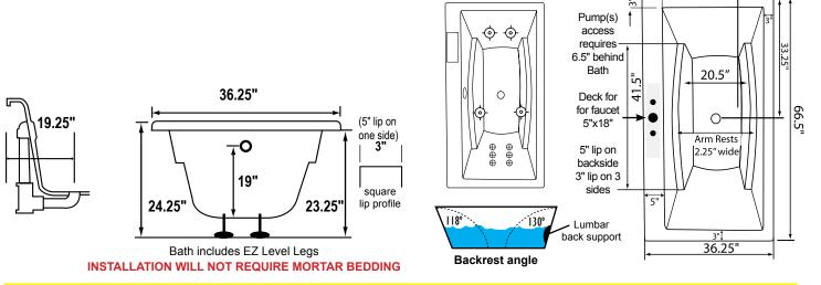
NOTE: Graphics may not be to scale. Specifications and features are subject to change without notice and are ± .25". All final measurements should be taken from tub on site. Access 12"x36" is provided on whirlpool systems baths. Consult your contractor for installation requirements.
