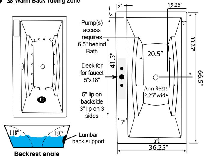
**NOTE: Graphics may not be to scale. Specifications and features are subject to change without notice and are ± .25". All final measurements should be taken from tub on site. Access 12"x36" is provided on whirlpool systems baths. Consult your contractor for installation requirements.**
